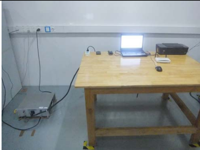
Conducted Emissions Test Setup – Front View
