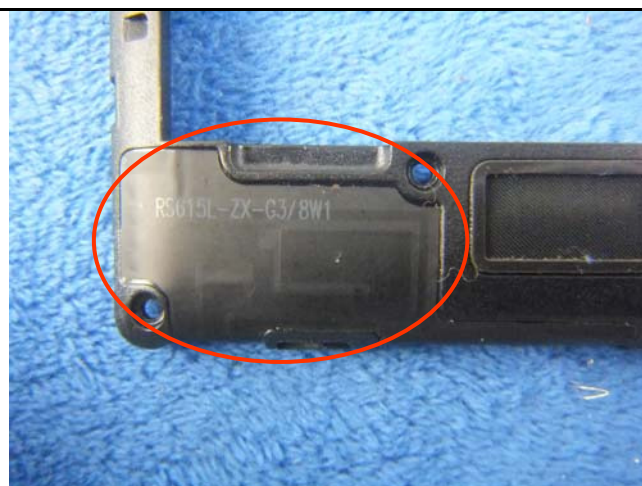
GSM/PCS/UMTS-FDD Antenna View
