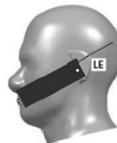
Picture17 Tilt position. The reference points for the right ear (RE), left ear (LE), and mouth (M), which define the Reference Plane for handset positioning, are indicated.
