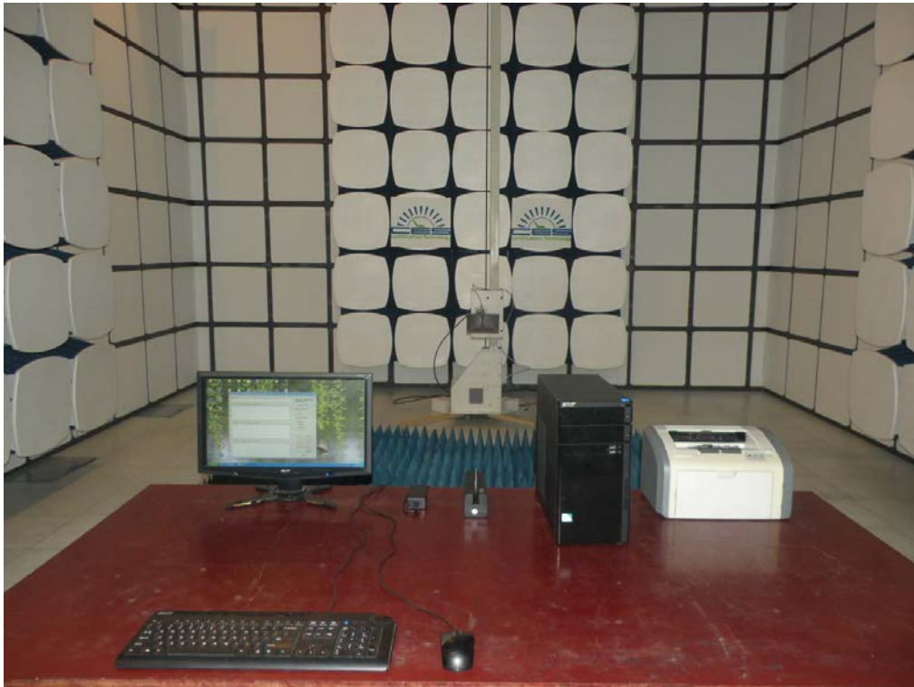
Photos of Power Line Conducted Emission Test
