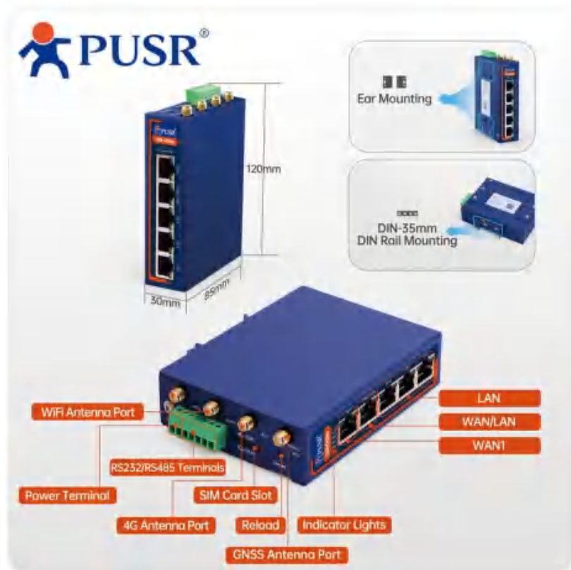
Pic 1 USR-G806p Product interface diagram
