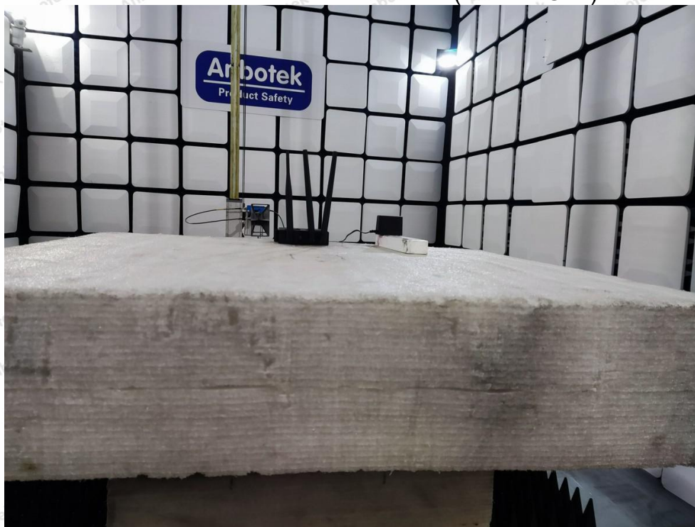
Photo of Radiation Emission Test (Above 1GHz)
