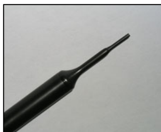
EX3DV4 E-field Probe
