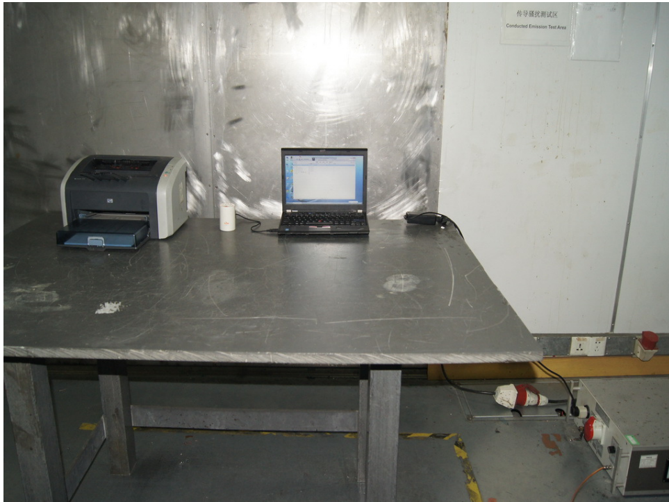
Photograph 6: Set-up for Radiated Emissions, below 1GHz
