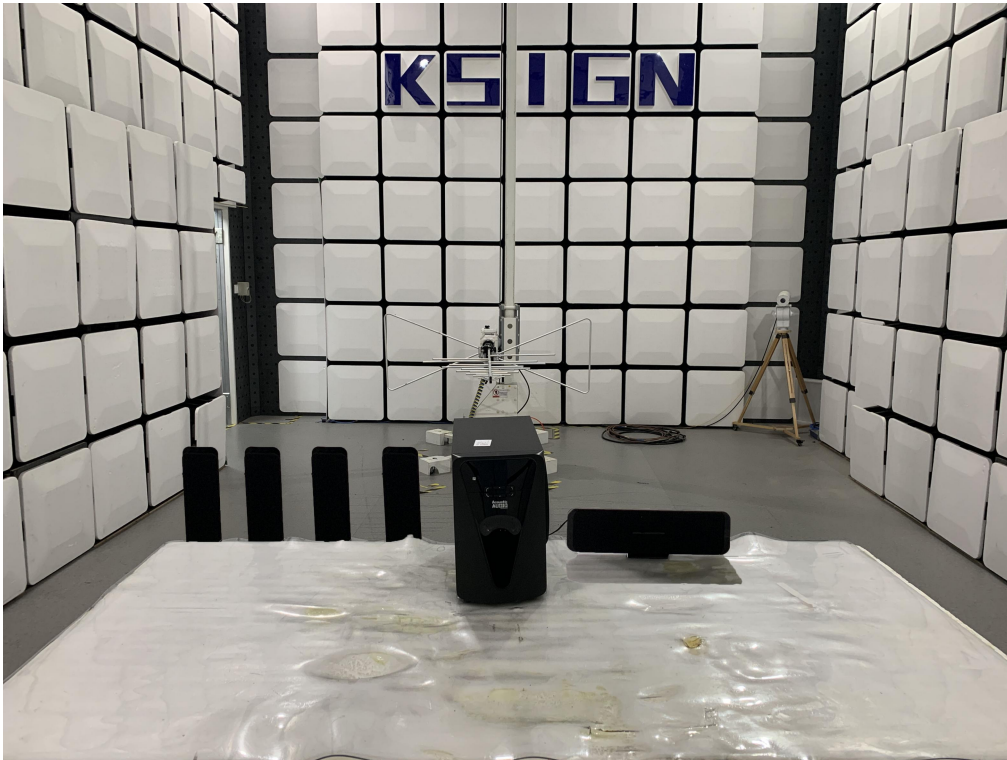
Radiated Measurement (Above 1GHz)
