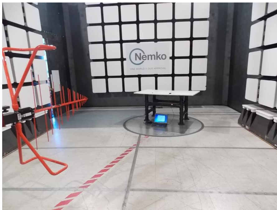
Figure 8.3-3: Radiated field strength setup photo
