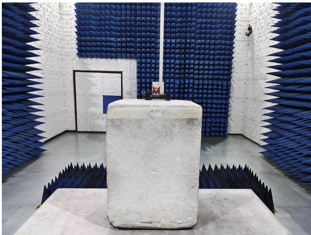
FCC RADIATED EMISSION TEST SETUP ABOVE 1GHZ
