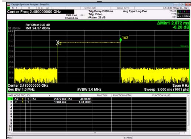
Pulse Width GFSK_DH5
