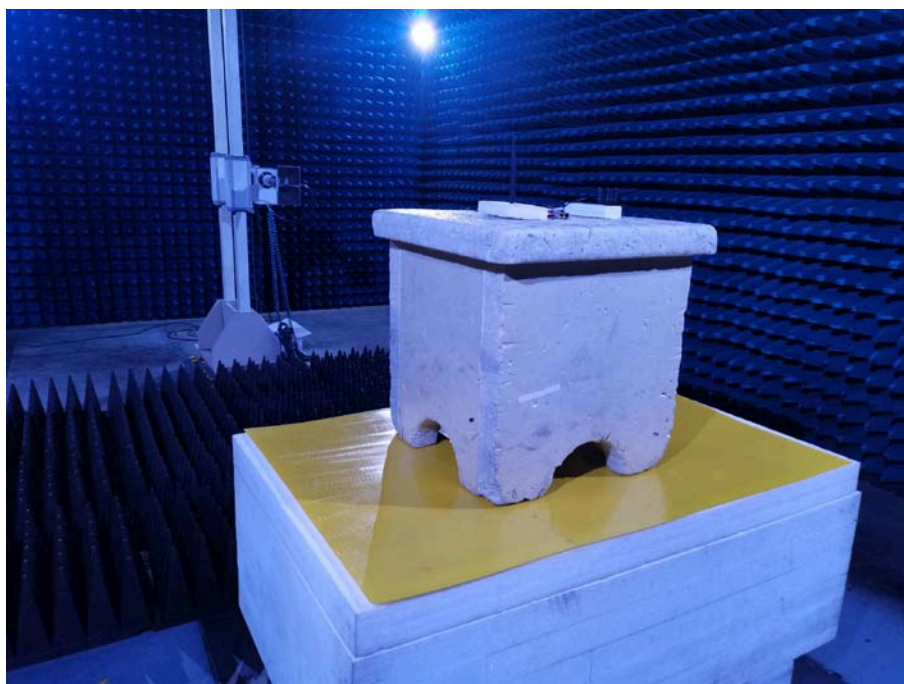
Photo of Radiated Emission Measurement Above 1GHz
