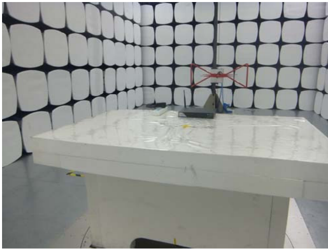
Radiated Spurious Emissions Test Setup Below 1GHz
