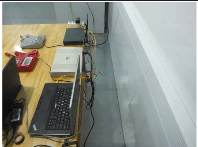
Conducted Emissions Test Setup Side View
