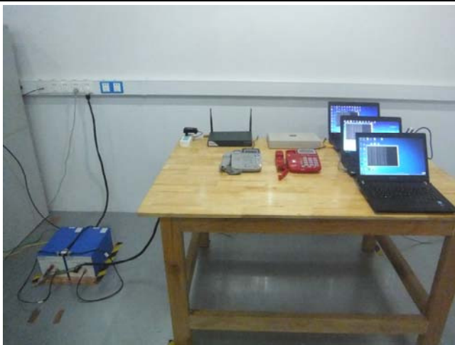
Conducted Emissions Test Setup Front View
