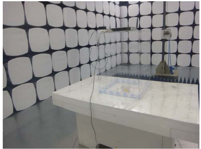
Radiated Spurious Emissions Test Setup Above 1GHz
