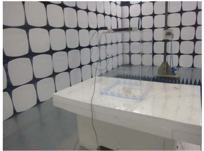
Radiated Spurious Emissions Test Setup Above 1GHz
