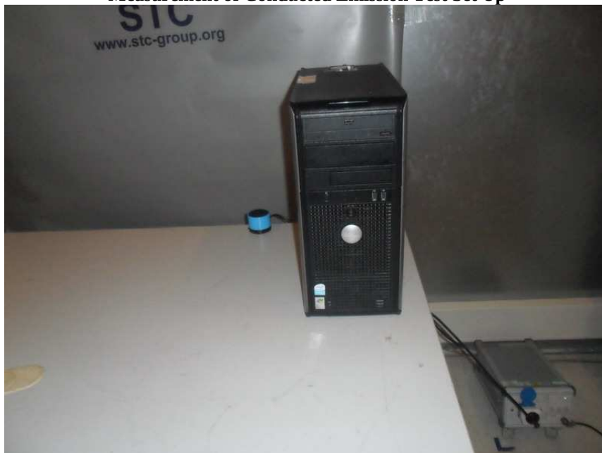
Measurement of Conducted Emission Test Set Up
