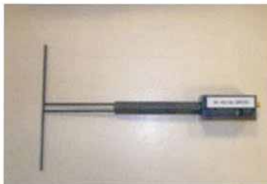
Figure 1 – Satimo COMOSAR Validation Dipole
