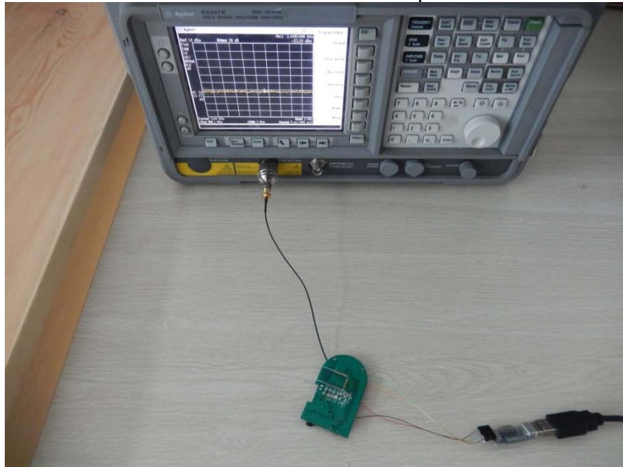
DSS&DTS RF conduction test photos
