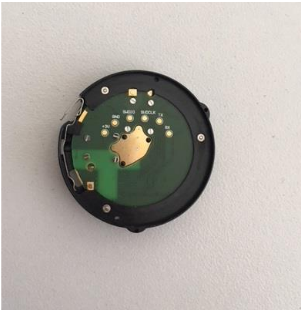
Photo 5: PCB back side view
