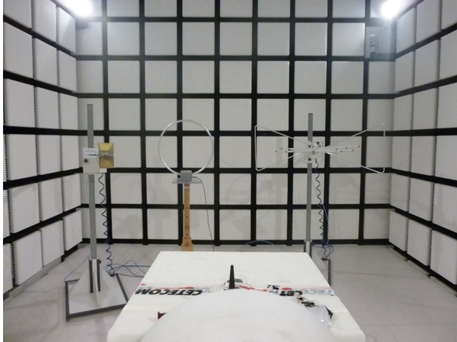
Photo 5: EUT at the anechoic chamber
