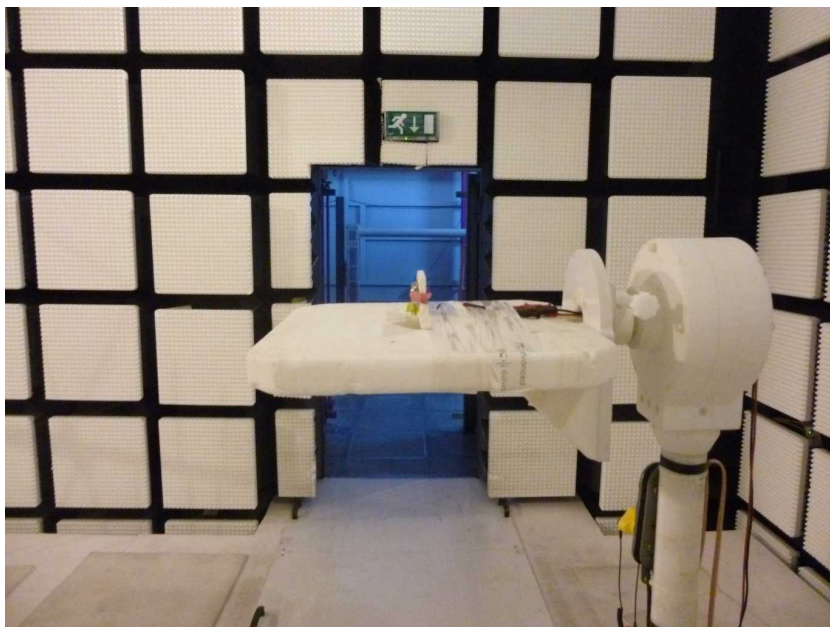
Photo 6: EUT at the anechoic chamber
