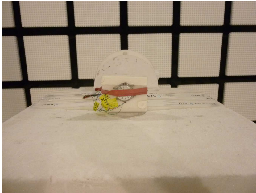
Photo 1: EUT at the anechoic chamber
