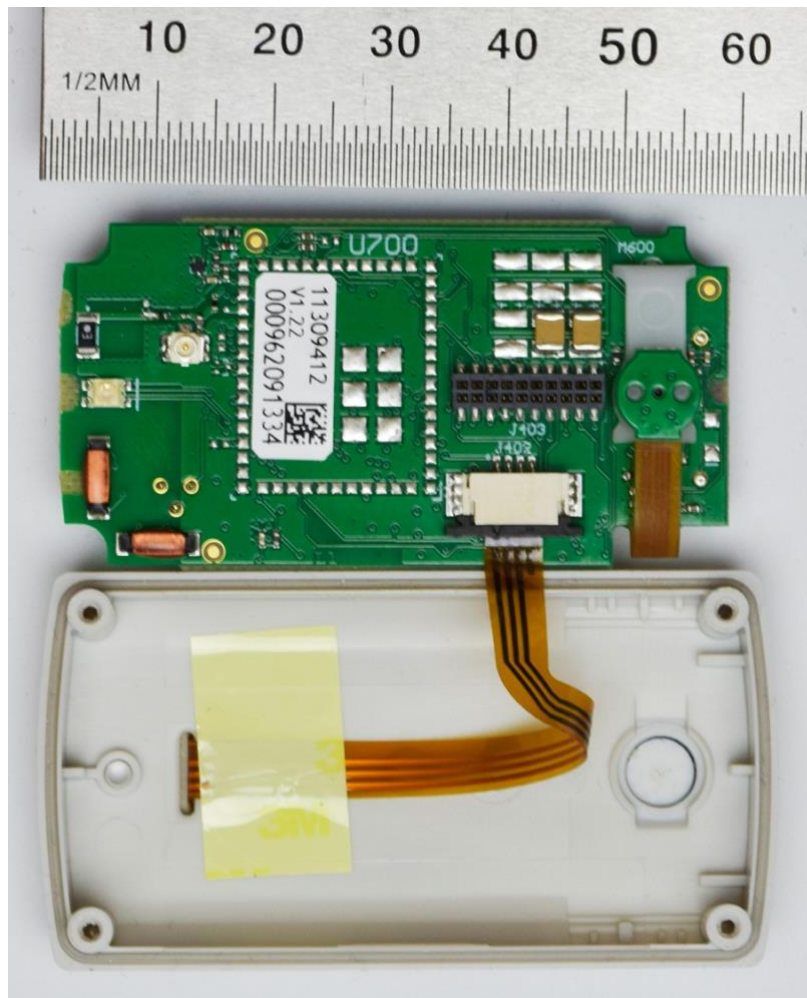
Figure 3: The inside of the top of the tag with the PBA lifted out and flipped.
