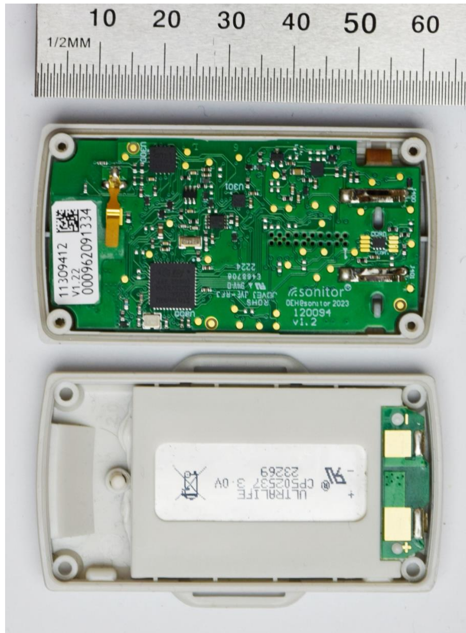
Figure 2: The inside of the top of Tag-M503 (upper part of the photo) and the base (lower part of the photo). The sub-assembly containing a thin-film battery is placed inside the housing of the base.
