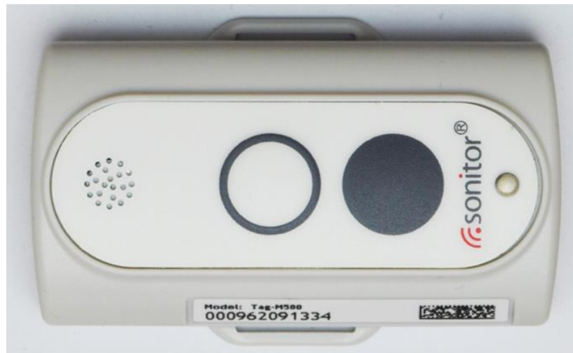
Figure 1: Photo of Tag-M500 where the color button (A) is seen to the left and the black button (B) to the right. An LED indicator is seen to the right of the Sonitor logo.
