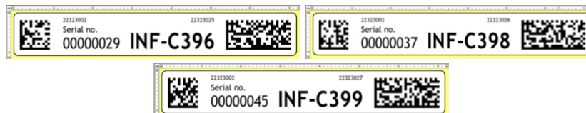
Figure 3: TAB ID labels, 57 x 11 mm 2 , with a Datamatrix to the left for the Serial no. and a Datamatrix to the right for the GIAI following GS-1.
