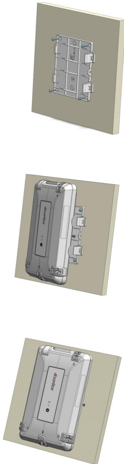
Figure 7: Illustration of how to mount to ceiling plates.
