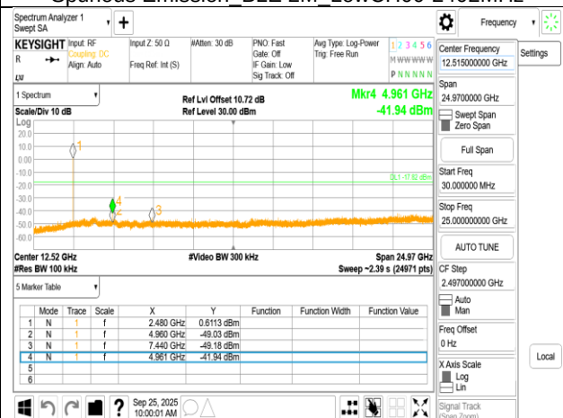
Spurious Emission_BLE 2M_HighCH39-2480MHz
