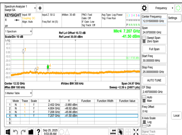
Spurious Emission_BLE 2M_LowCH00-2402MHz
