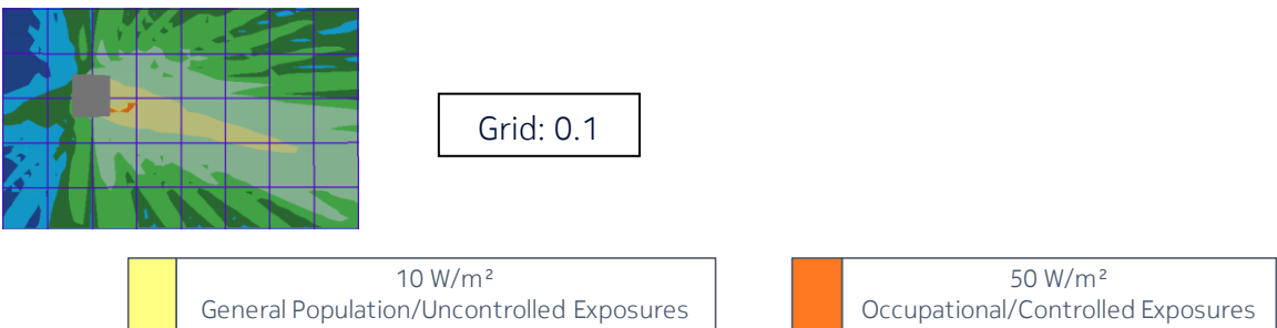
Figure 6 – Side view of the power density for the time-averaged actual maximum transmitted power of 0.283 W and the beam oriented in azimuth = 0° & elevation = +15°
