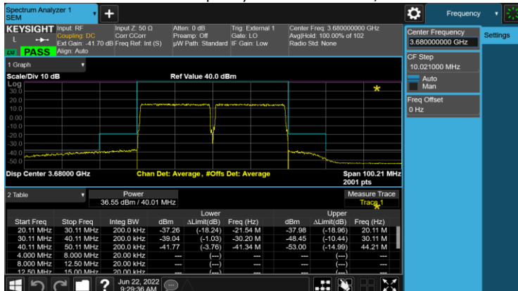
Test Model 3.1a, Modulation 256QAM, Channel Frequency 3670 + 3690 MHz, TX1
