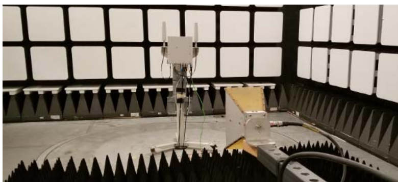
Figure 5. Setup Photos of Radiated Test for AZRB with Various Antennas (BA-AIO3O3T3T3VJX65F-06, PAS2457-CC1, GO4806-06664, 2205 & FA2RA)
