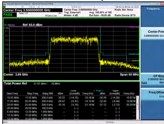
OBW 1 Carrier 20MHz 256QAM 3690 MHz
