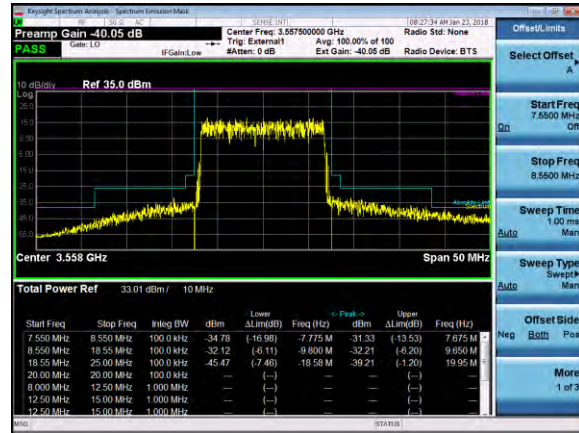
OBW 1 Carrier 15MHz 256QAM 3557.5 MHz
