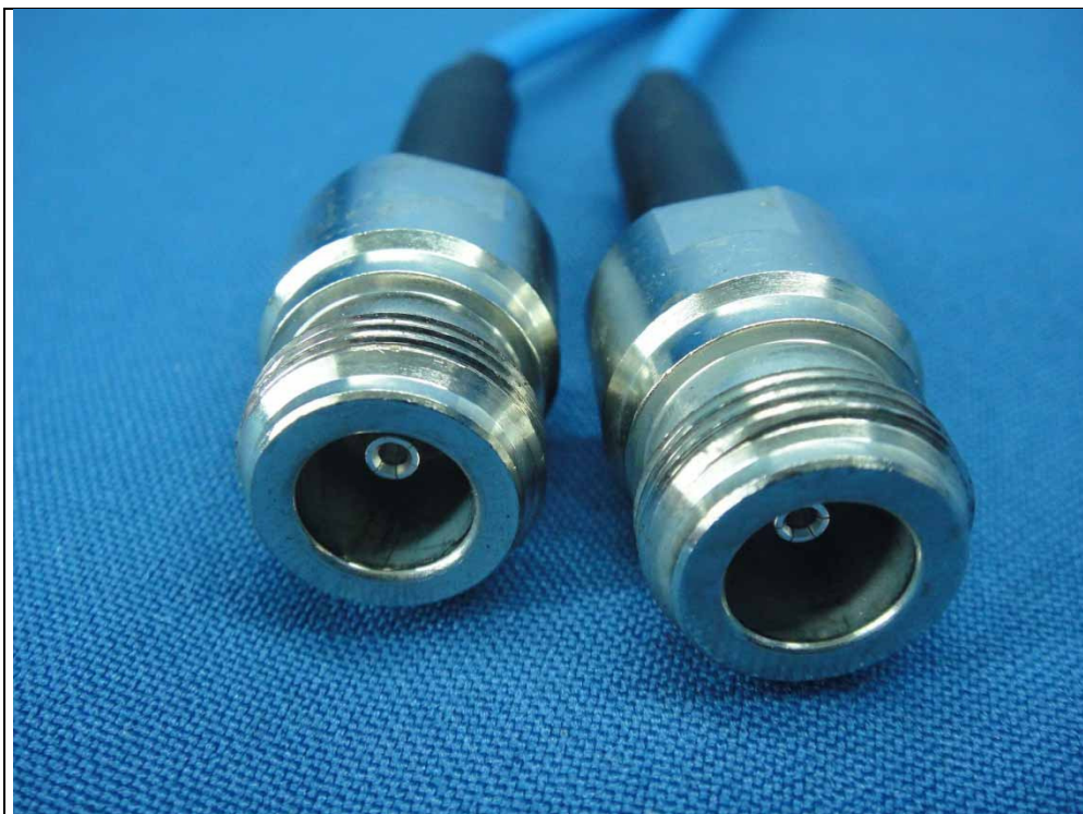
LTE external antenna cable connector
