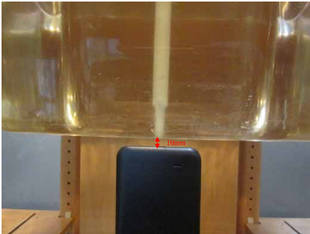
Body-worn Bottom Setup Photo (10mm)
