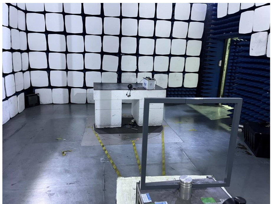
Radiation Emission Test Setup (Below 30MHz)
