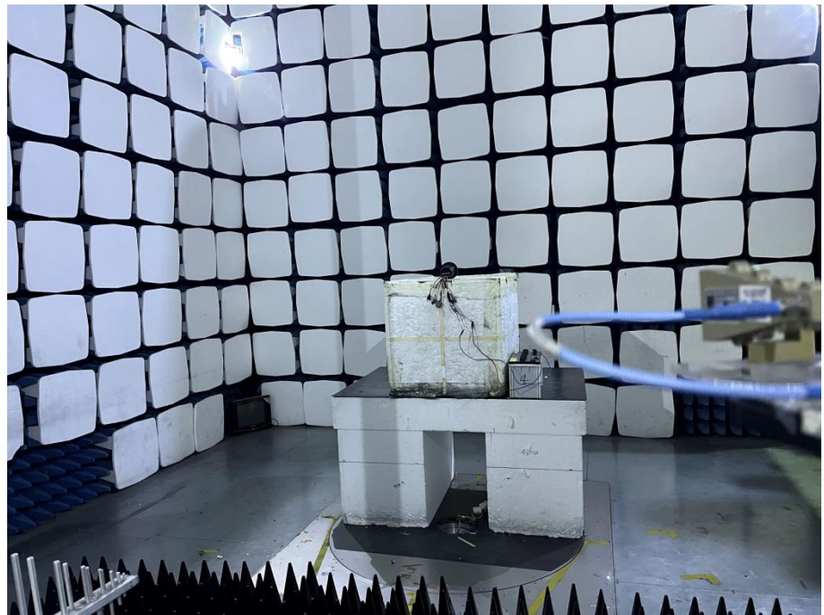
Radiation Emission Test Setup (Above 18GHz)
