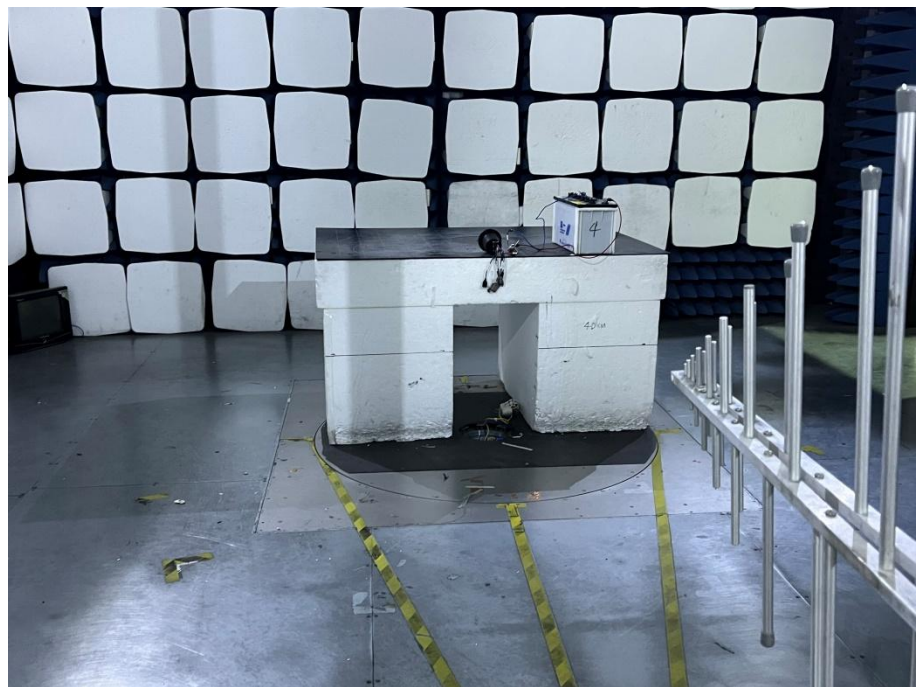
Radiation Emission Test Setup (30MHz to 1GHz)
