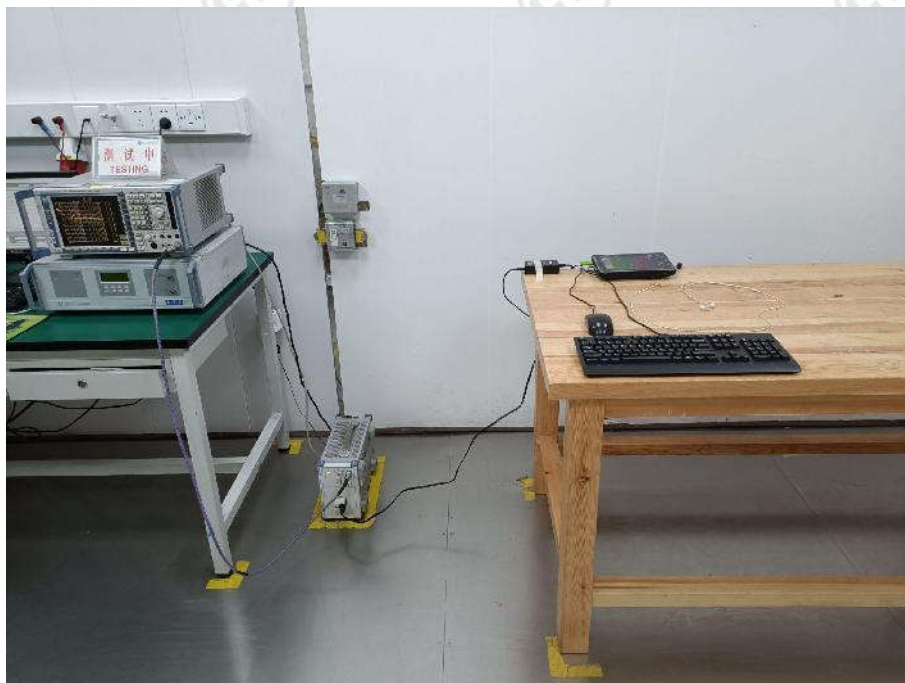
Conducted Emissions Test Setup
