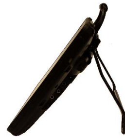
Stand latched in the fully extended position
