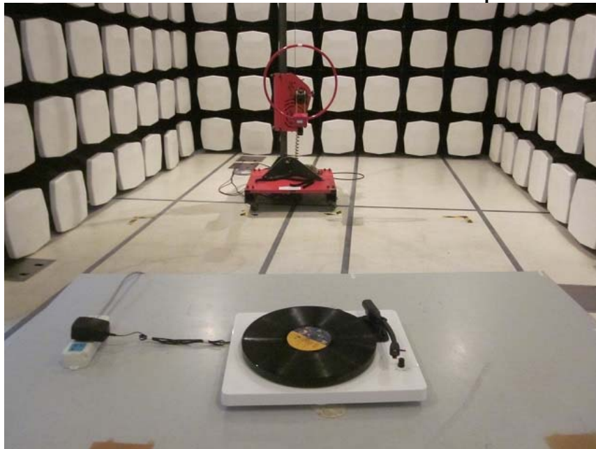
Measurement of Radiated Emission Test Set Up
