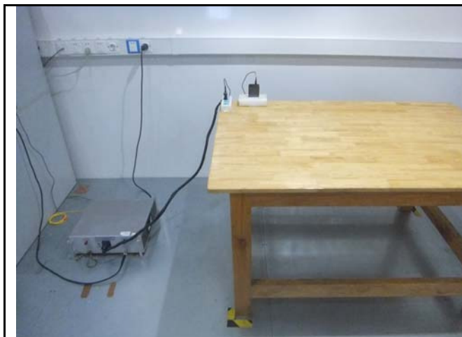
Conducted Emissions Test Setup Front View
