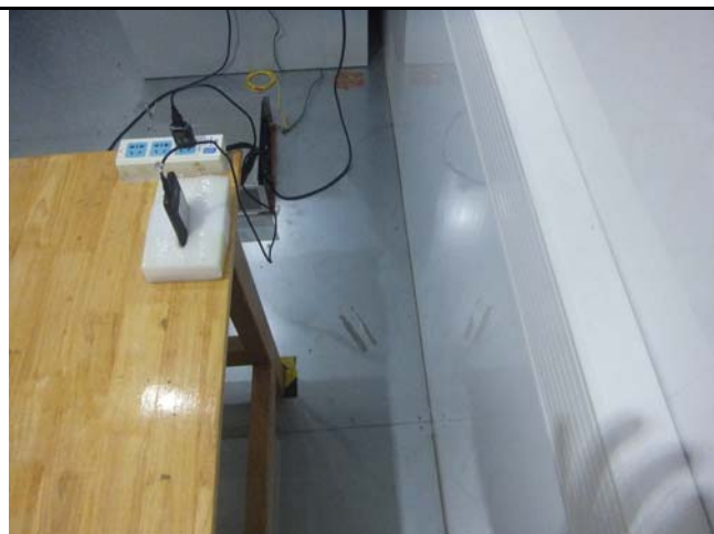
Conducted Emissions Test Setup Side View
