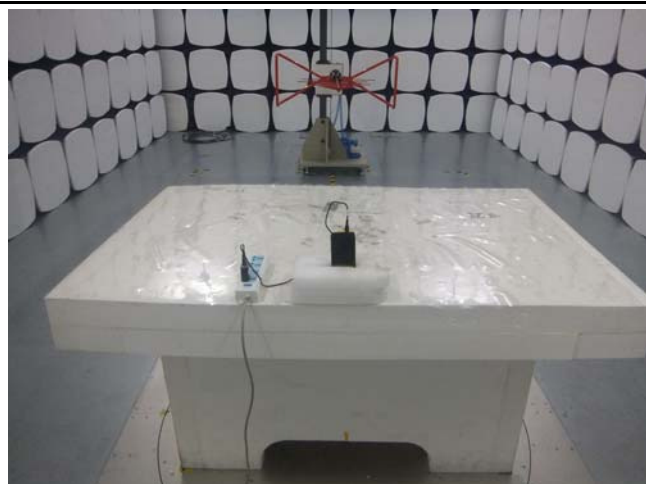
Conducted Emissions Test Setup Front View
