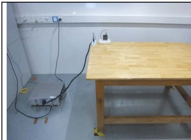
Conducted Emissions Test Setup Front View
