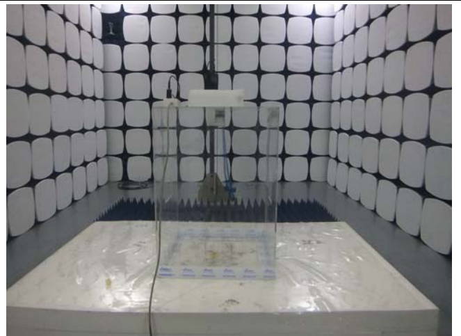
Radiated Spurious Emissions Test Setup Above 1GHz
