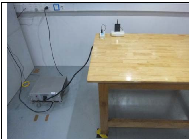
Conducted Emissions Test Setup Front View
