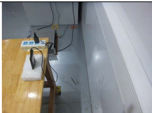
Conducted Emissions Test Setup Side View
