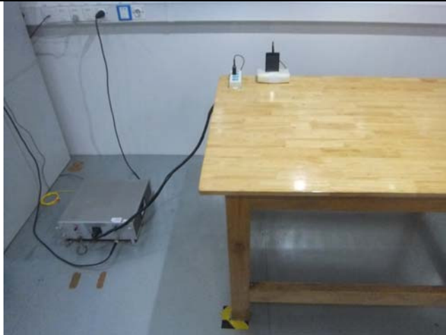
Conducted Emissions Test Setup Front View
