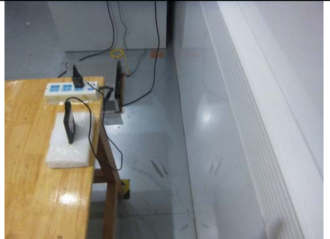
Conducted Emissions Test Setup Side View
