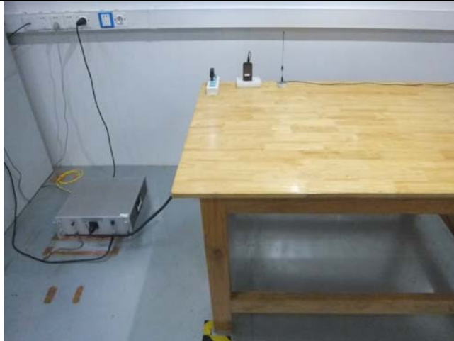
Conducted Emissions Test Setup Front View
