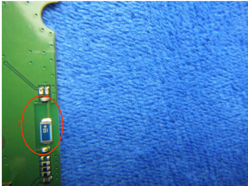
BT - Antenna View
