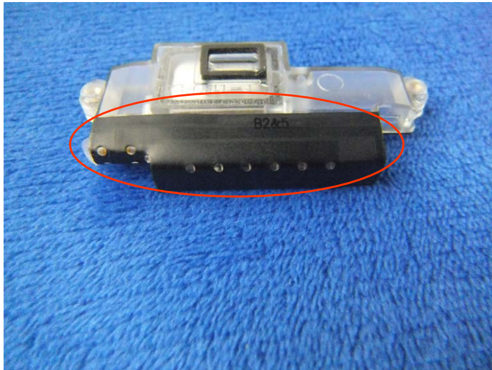
GSM/PCS/UMTS-FDD Antenna View
