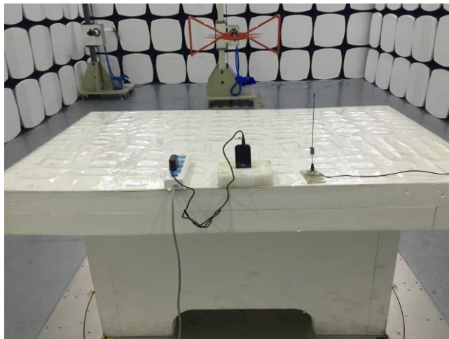
Radiated Spurious Emissions Test Setup Below 1GHz
