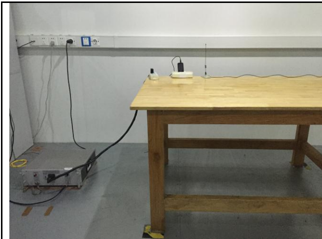
Conducted Emissions Test Setup Front View
