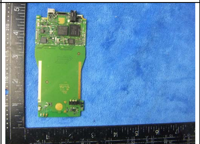
Mainboard without Shielding - Front View
