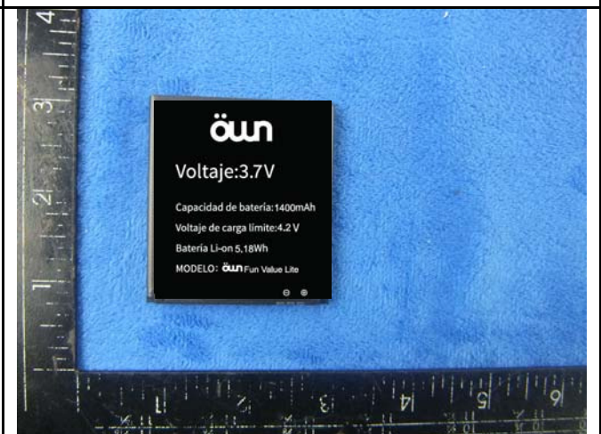
Battery - Rear View
