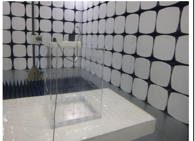
Radiated Spurious Emissions Test Setup Above 1GHz
