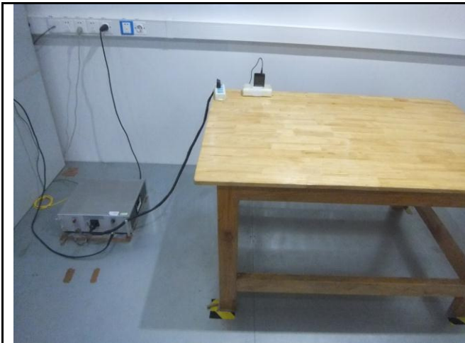
Conducted Emissions Test Setup Front View
