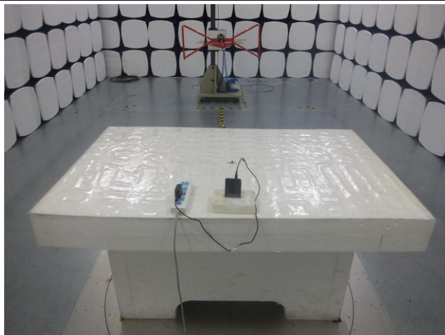
Conducted Emissions Test Setup Front View
