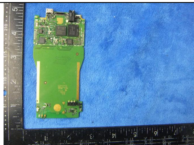
Mainboard without Shielding - Front View
