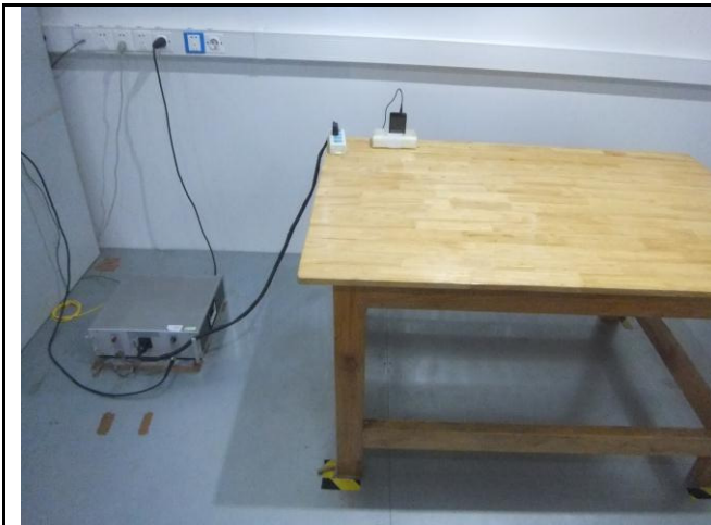
Conducted Emissions Test Setup Front View
