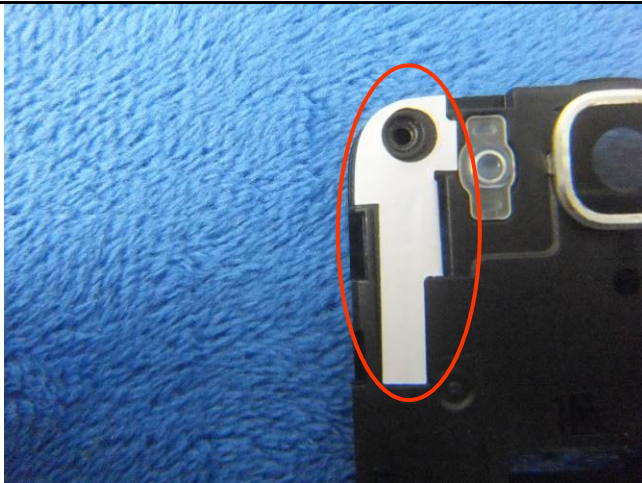
LTE Antenna View
