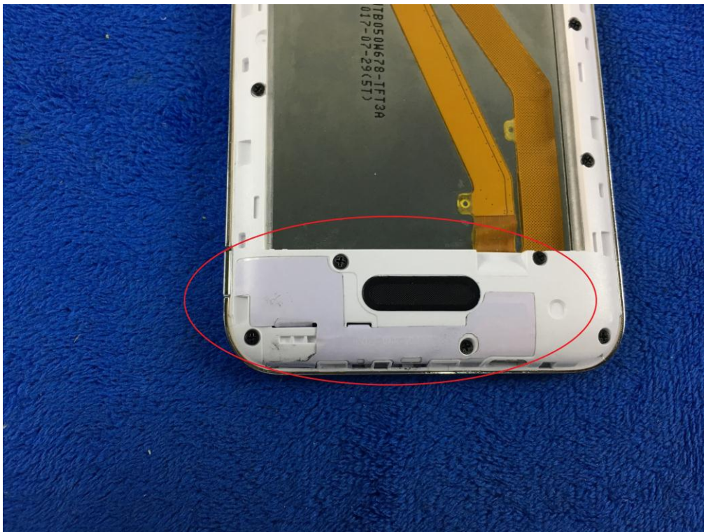
GSM/PCS/UMTS-FDD Antenna View
